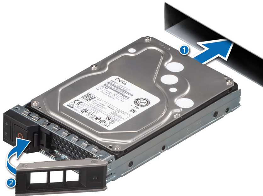
Figure 45. Installing a drive carrier
