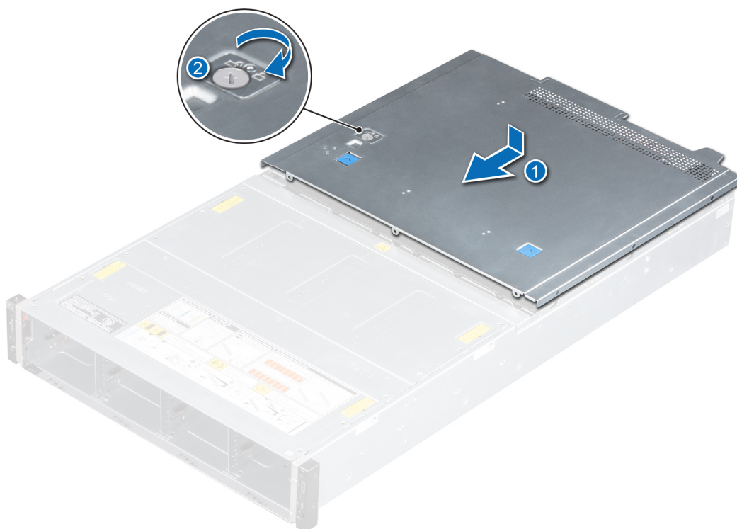
Figure 22. Installing system cover
