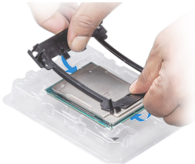
Figure 78. Installing the processor bracket
