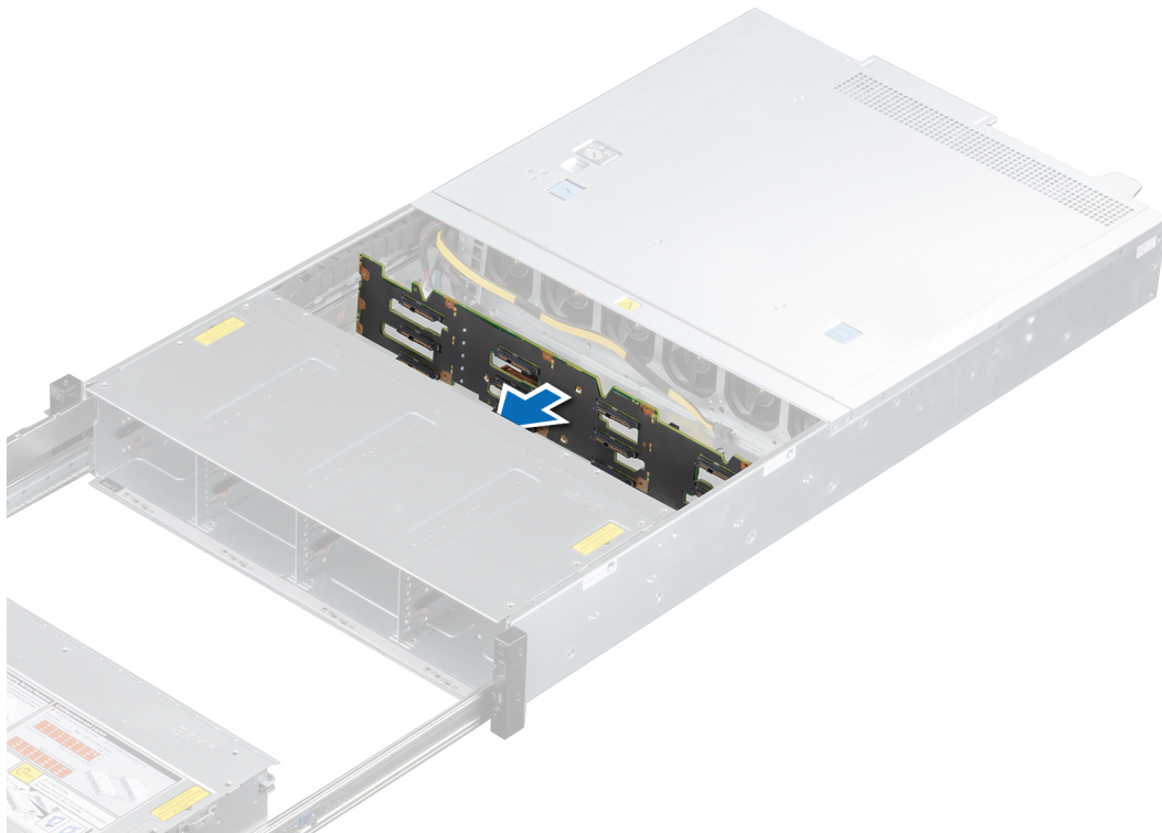
Figure 66. Installing bay 2 backplane
