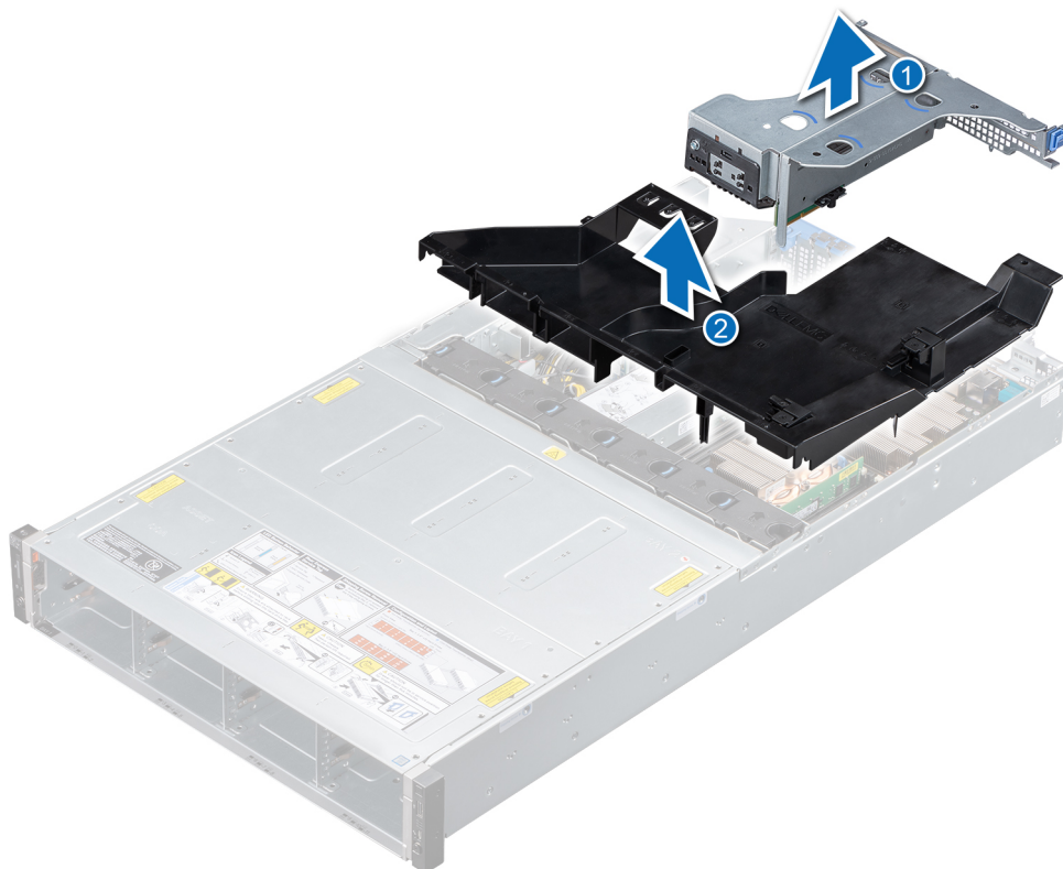
Figure 23. Removing air shroud
