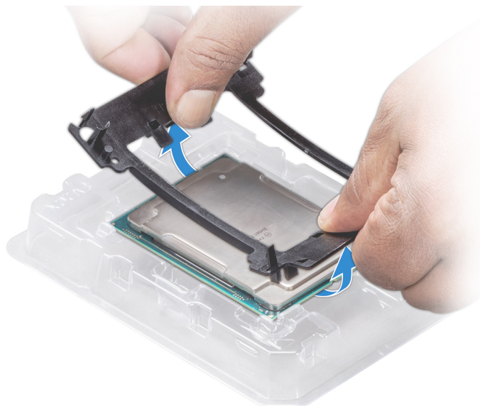
Figure 77. Removing the processor bracket
