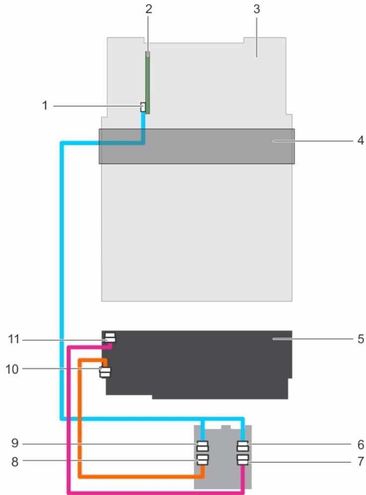
**Figure 91. Cabling—2.5 inch (x24) SAS/SATA backplane with PERC 9**
