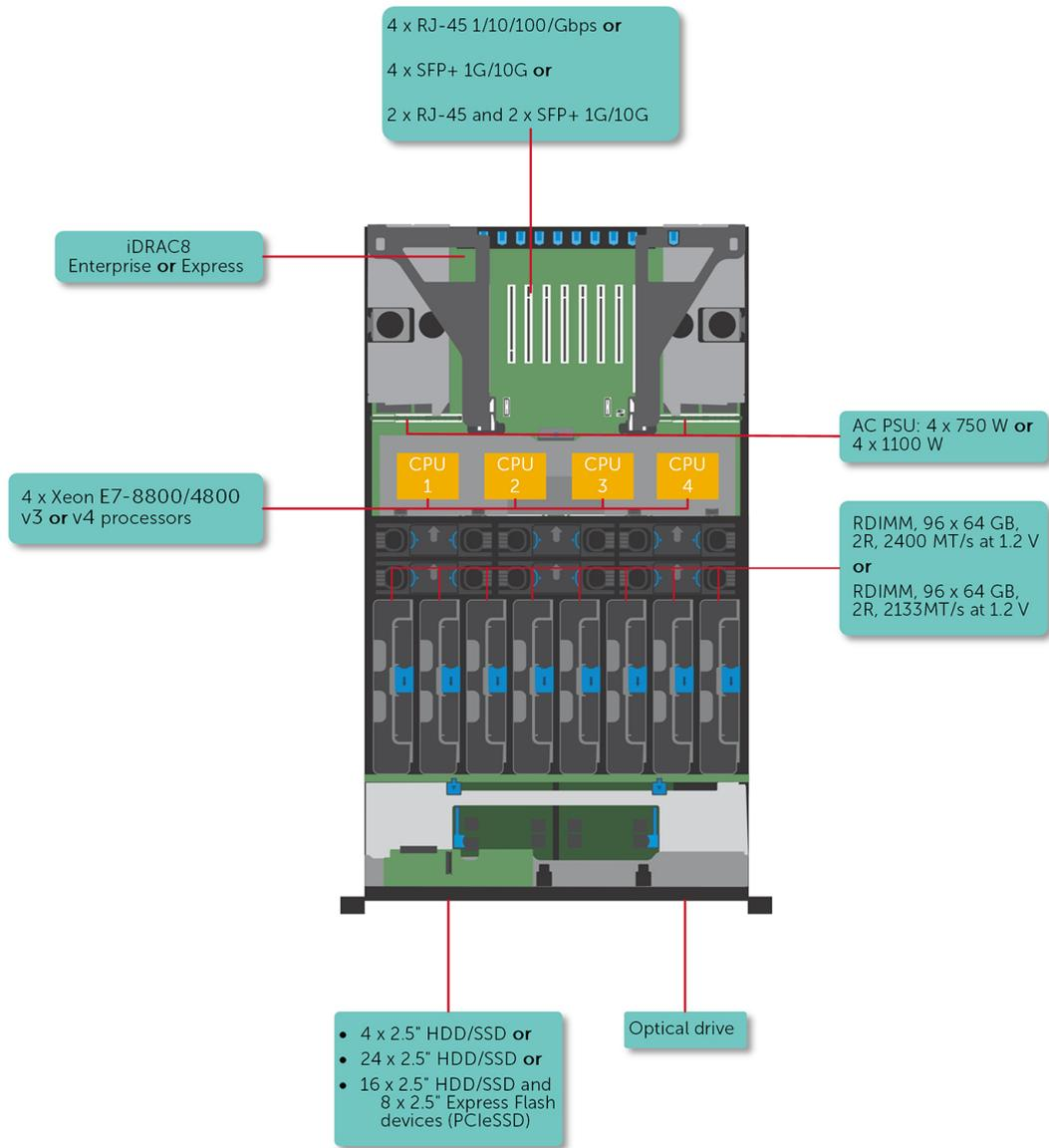
**Figure 1. Supported configurations for the PowerEdge R930 system**
