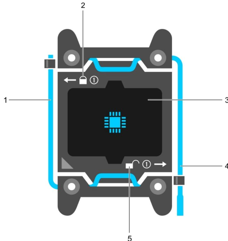
**Figure 70. Processor shield**
