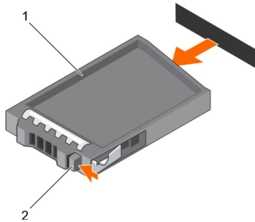
**Figure 35. Removing a 2.5-inch hard drive blank**
