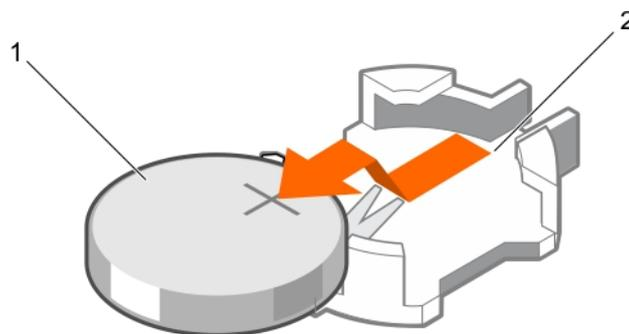
**Figure 85. Removing the system battery**
