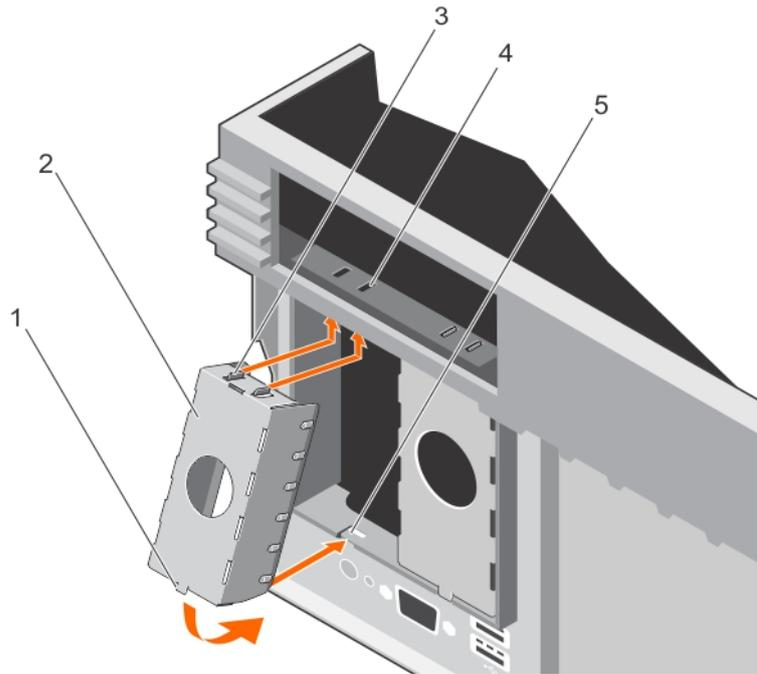
**Figure 80. Installing the PSU blank**
