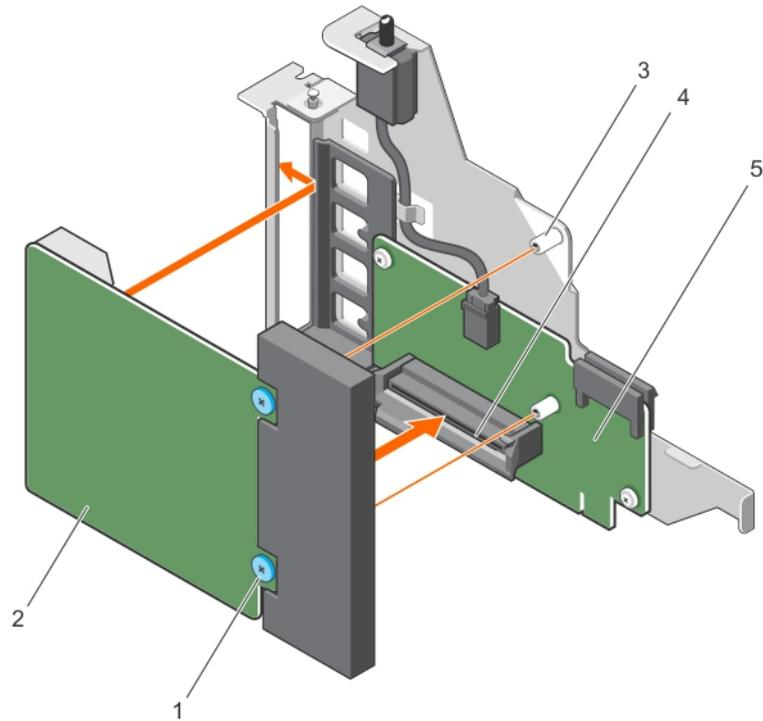
**Figure 59. Installing the NDC**
