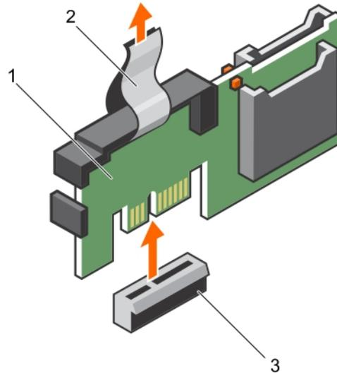
**Figure 65. Removing the internal dual SD module (IDSDM)**
