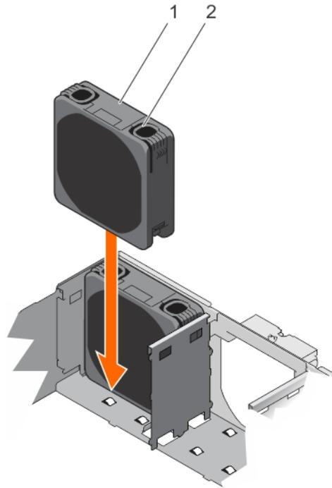
**Figure 28. Installing a cooling fan**
