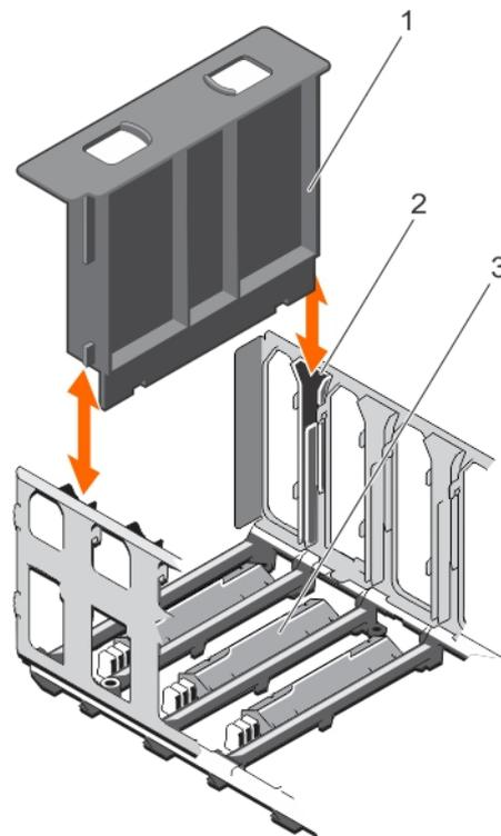
**Figure 17. Removing the memory riser blank**
