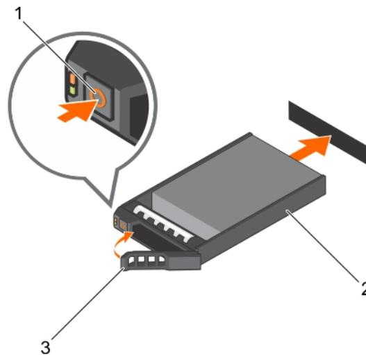
**Figure 38. Installing a hot swappable hard drive carrier**
