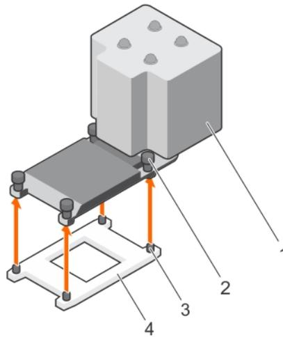
**Figure 69. Removing the heat sink**
