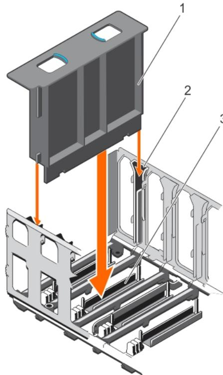
**Figure 18. Installing the memory riser blank**
