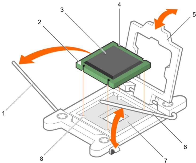
**Figure 72. Installing a processor**
