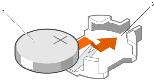
**Figure 86. Installing the system battery**
