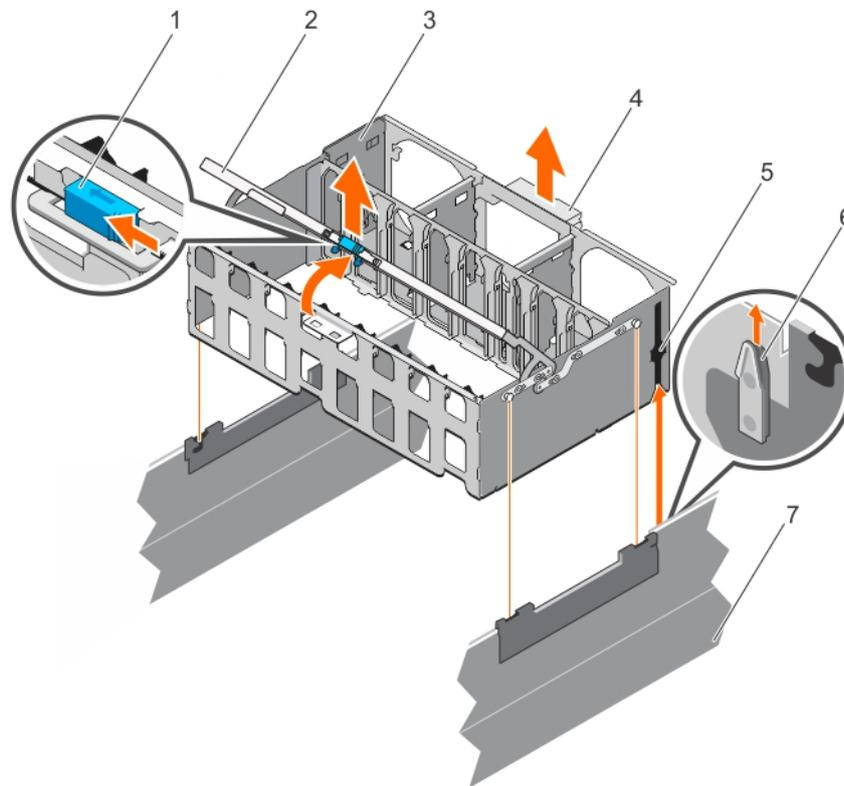
**Figure 25. Removing the memory riser and fan cage**
