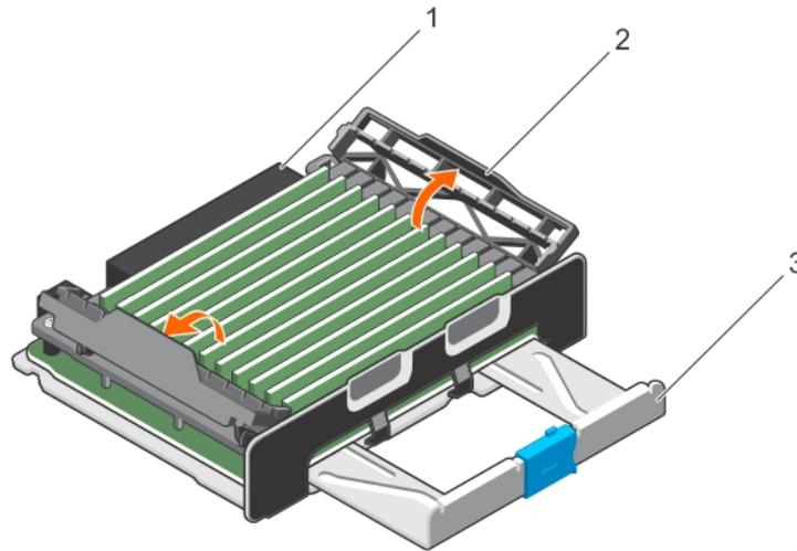
**Figure 21. Opening the memory riser**
