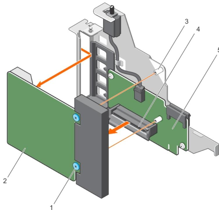
**Figure 58. Removing the NDC**
