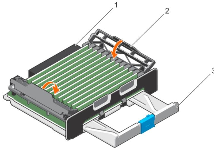
**Figure 24. Closing the memory riser**
