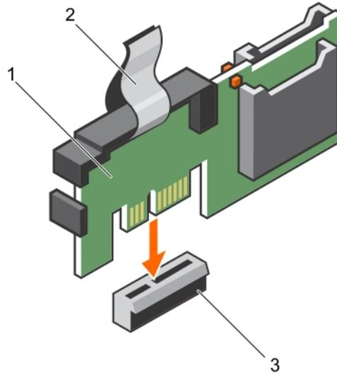
**Figure 66. Installing the optional internal dual SD module**
