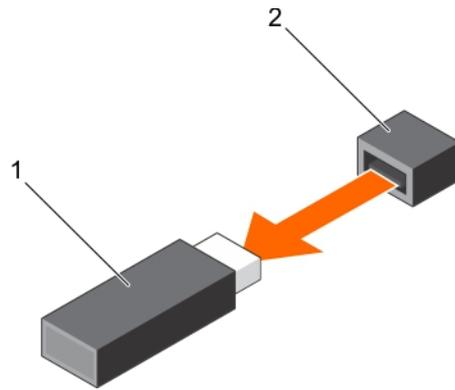
**Figure 43. Removing the internal USB memory key**
