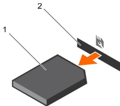
**Figure 62. Removing the optional SD vFlash card**
