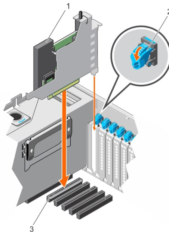
**Figure 57. Installing the NDC riser**
