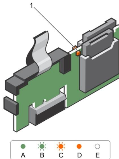
**Figure 9. Internal dual SD module (IDSDM)**
