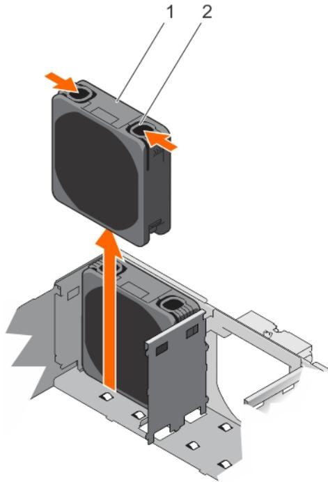
**Figure 27. Removing a cooling fan**
