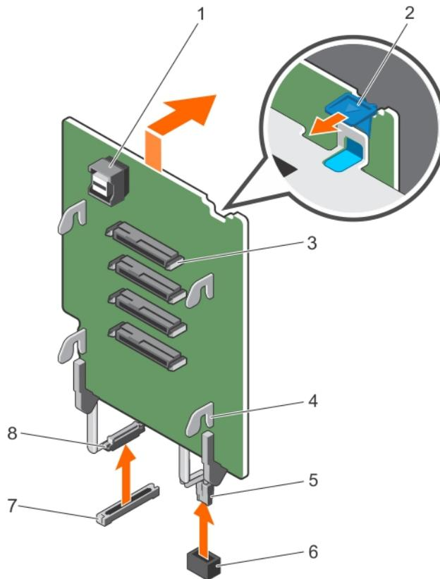
**Figure 87. Removing the 2.5 inch (x4) SAS/SATA backplane**
