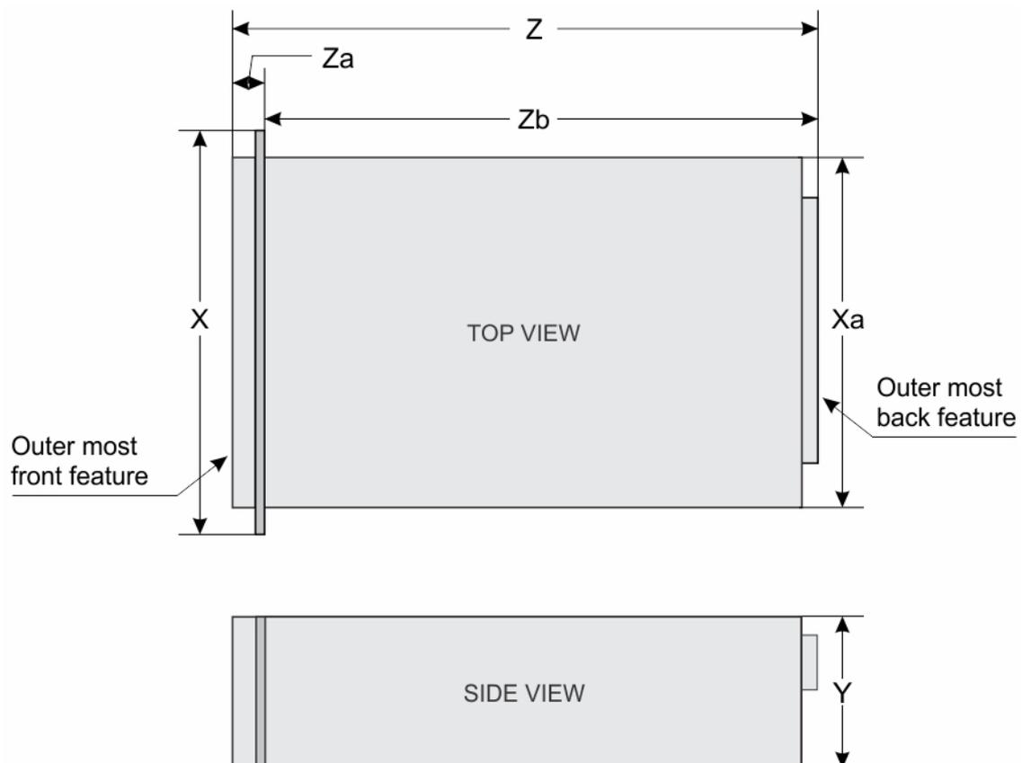
Figure 10. Chassis dimensions of the PowerEdge R930 system
