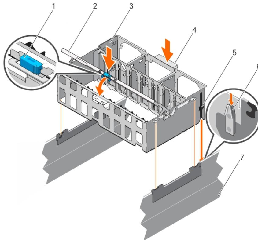
**Figure 26. Installing the memory riser and fan cage**
