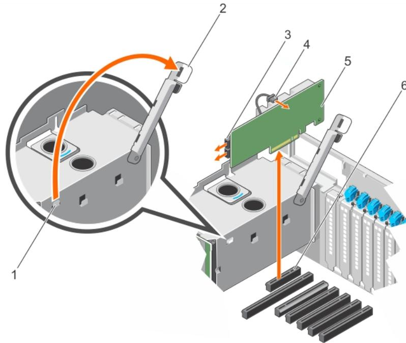
**Figure 67. Removing the integrated storage controller card**
