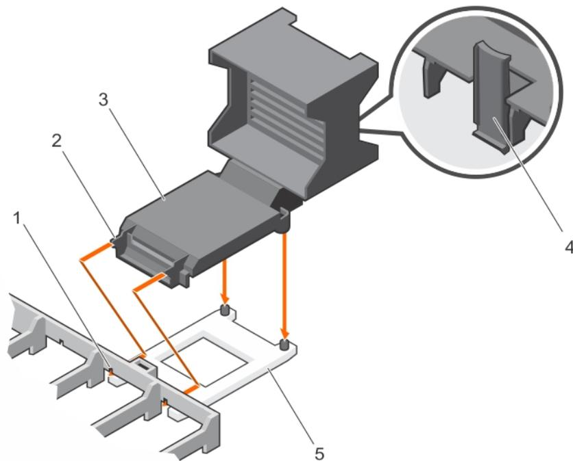
**Figure 76. Installing the processor and heat sink blank**
