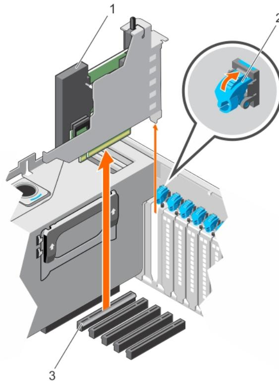
**Figure 56. Removing the NDC riser**
