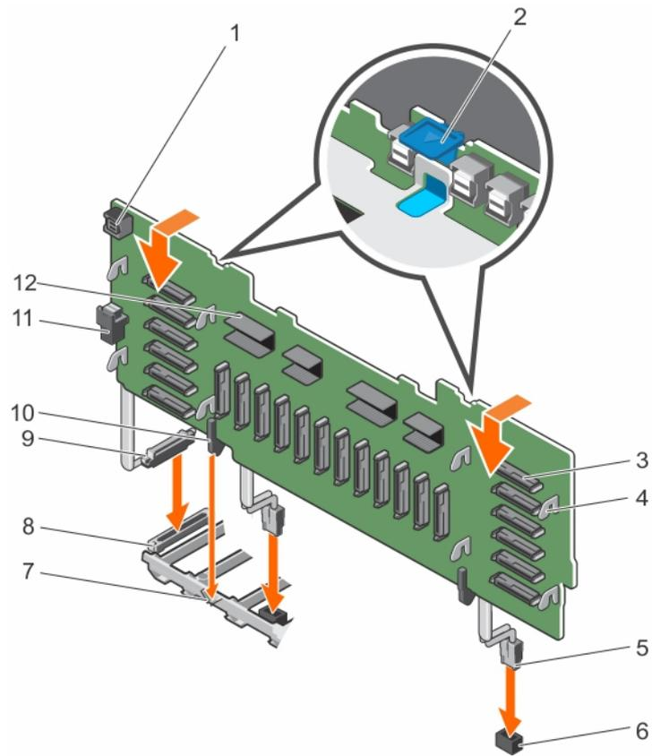
**Figure 95. Installing the 2.5 inch (x24) SAS/SATA backplane**
