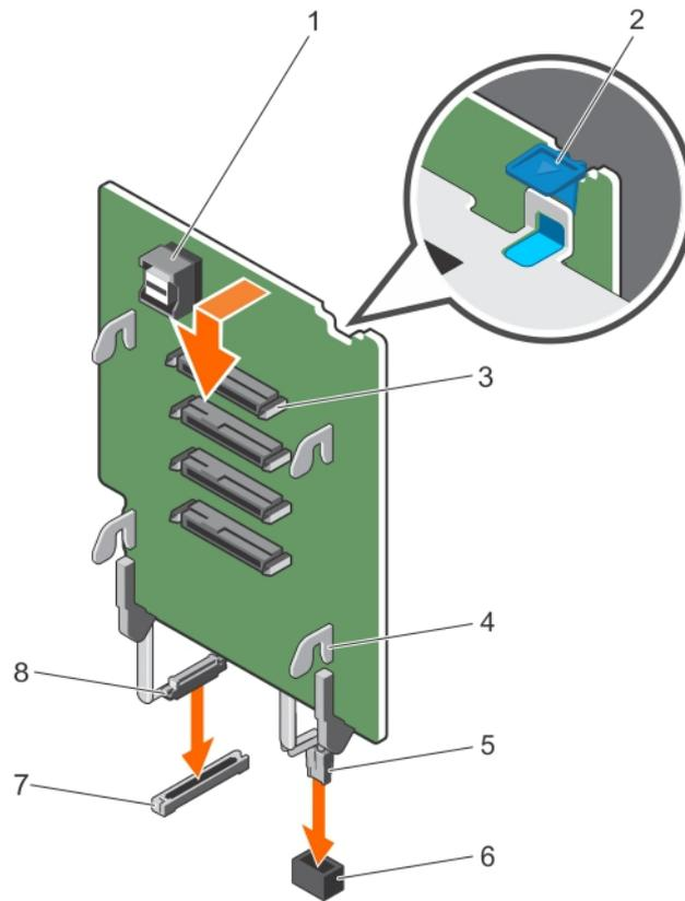
**Figure 94. Installing the 2.5 inch (x4) SAS/SATA backplane**
