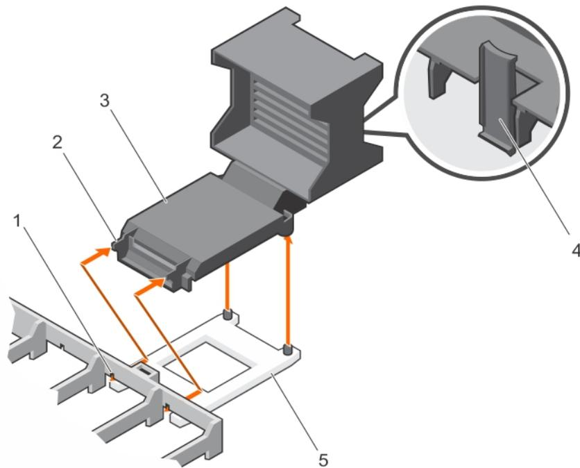
**Figure 75. Removing the processor and heat sink blank**
