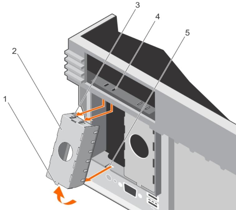
**Figure 79. Removing the PSU blank**
