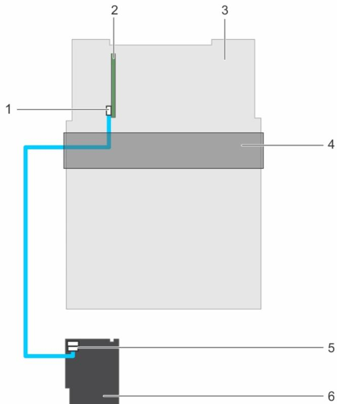
**Figure 90. Cabling—2.5 inch (x4) SAS/SATA backplane with PERC 9**
