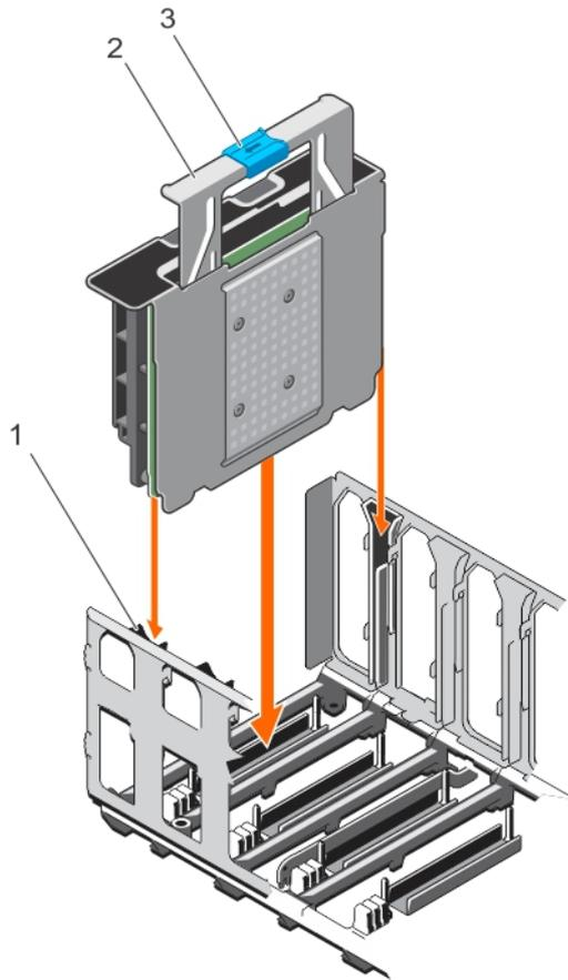
**Figure 20. Installing the memory riser**
