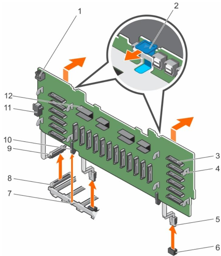
**Figure 88. Removing the 2.5 inch (x24) SAS/SATA backplane**
