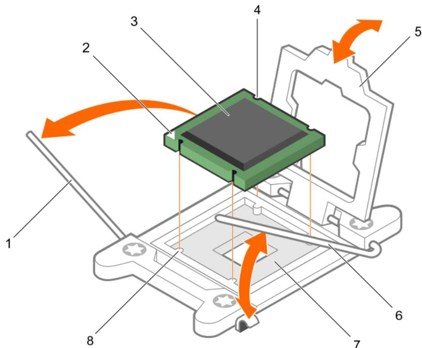
**Figure 71. Removing a processor**
