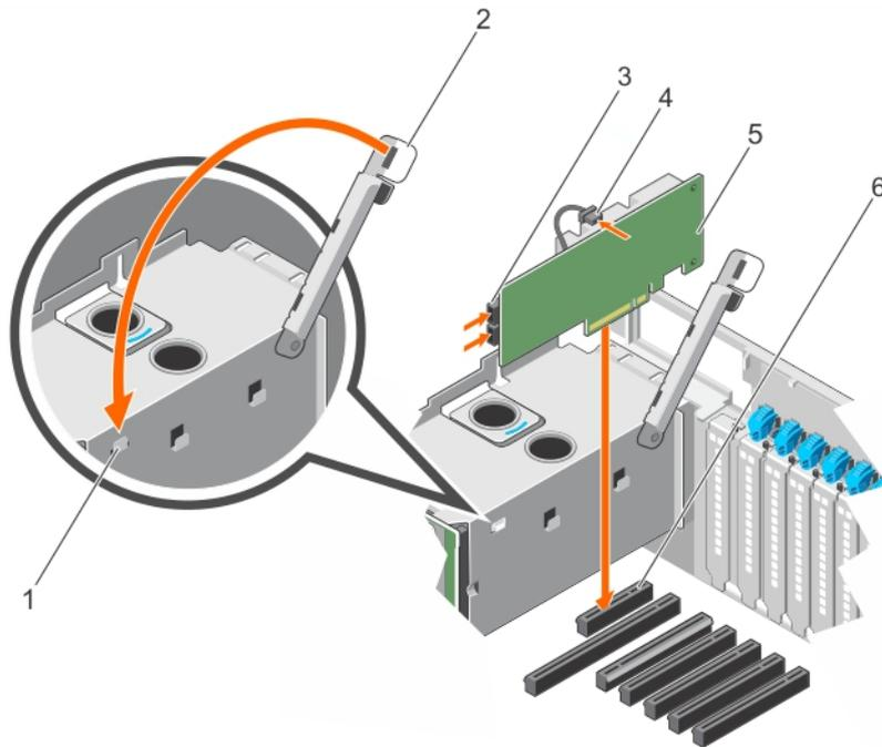
**Figure 68. Installing the integrated storage controller card**
