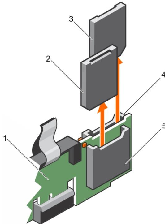
**Figure 63. Removing an internal SD card**
