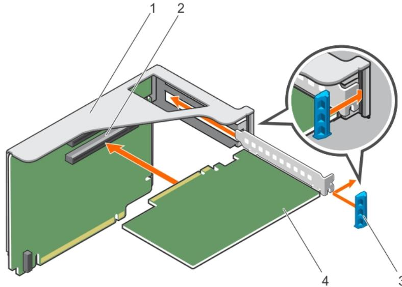
**Figure 55. Installing the expansion card from the right expansion card riser**
