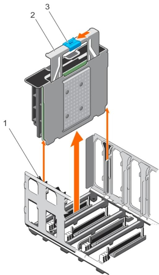
**Figure 19. Removing the memory riser**
