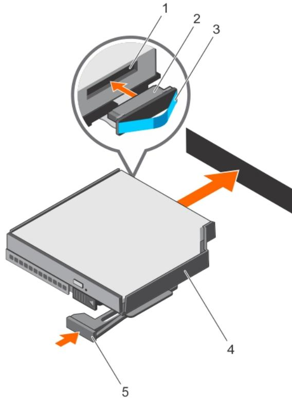
**Figure 42. Installing the optical drive**
