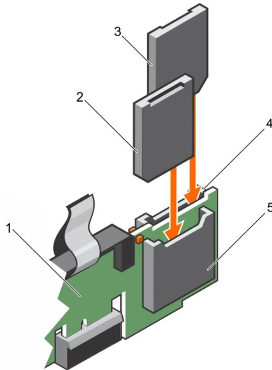
**Figure 64. Installing an internal SD card**
