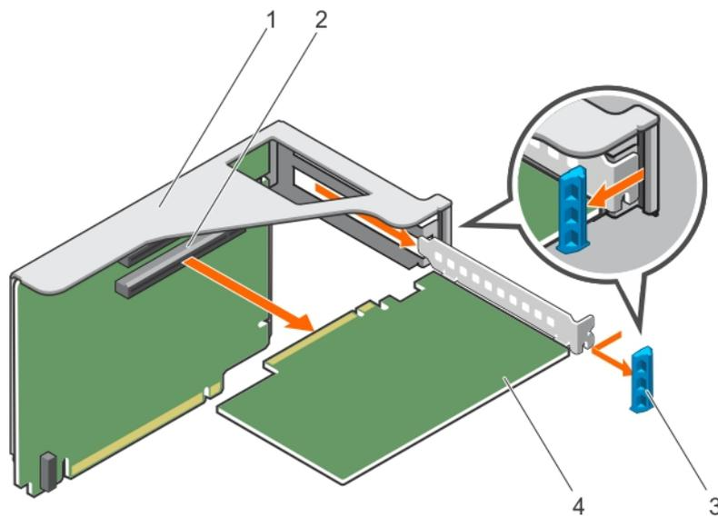
**Figure 51. Removing the expansion card from the right expansion card riser**
