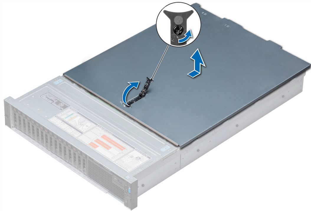
Figure 26. Removing the system cover
