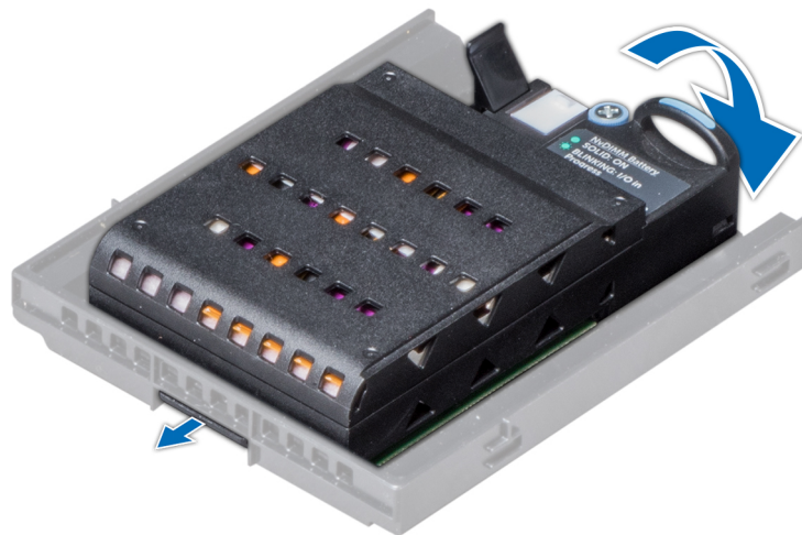
Figure 45. Installing NVDIMM-N battery into the bracket
