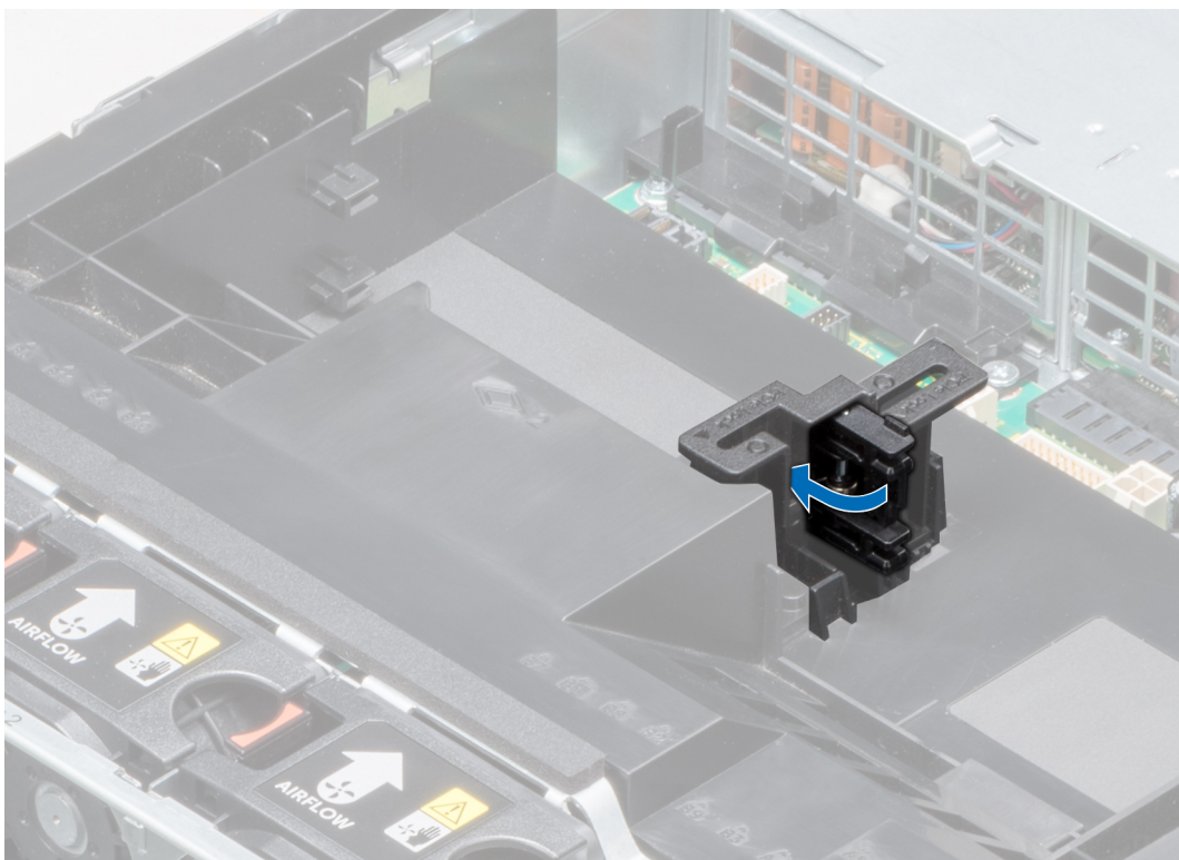
Figure 82. Closing the PCIe card holder latch
