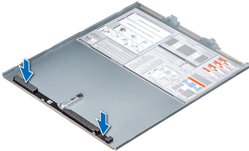
Figure 114. Installing mylar foam on the system cover
