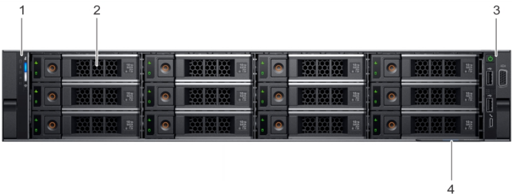
Figure 3. Front view of 12 x 3.5 inch drive system
