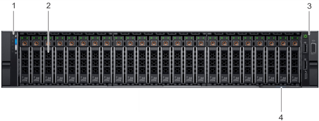
Figure 2. Front view of 24 x 2.5 inch drive system
