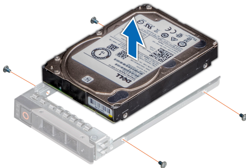
Figure 64. Removing the drive from the drive carrier
