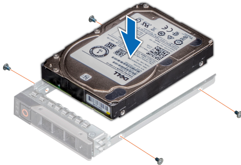
Figure 65. Installing a drive into the drive carrier
